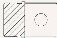
M1 = Type M, M12 thread, depth 20 mm
