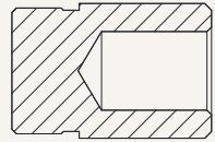
M2 = Type M, M14 thread, depth 20 mm
