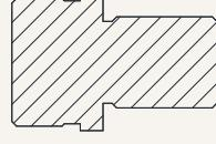
L1 = L shape, width 6mm, aperture 6.1mm
