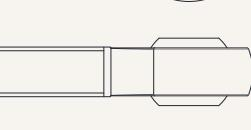
G1 = Spherical bearing, bore 12mm, model GS12
