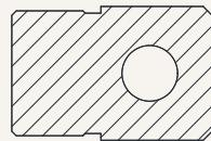
U1 = groove width 8.1mm, hole diameter 6.1mm
