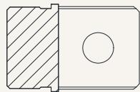
U2 = groove width 8.1mm, hole diameter 8.1mm
