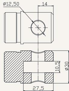
U2 =U-type, groove width 6.1mm, Aperture 10.5mm
