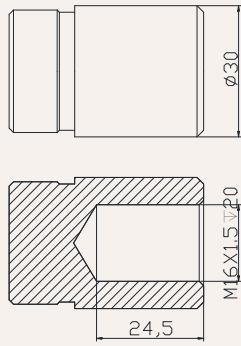
M2 = Type M, M30 thread, depth 20 mm
