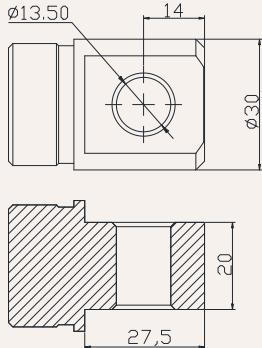
G1 = Spherical bearing, bore 20mm, model GS20
