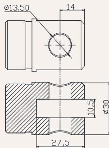
M1 = Type M, M25 thread, depth20 mm
