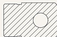
L2 = L shape, width 20mm, aperture 13.5mm
