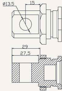
G1 = Spherical bearing, bore 14mm, model GS14
