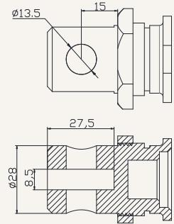
M1 = Type M, M18 thread, depth 20 mm
