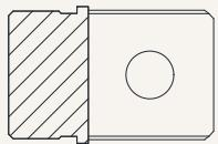
U2 = groove width 10.1mm, hole diameter 13.5mm
