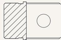
M1 = Type M, M18 thread, depth 20 mm
