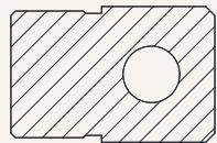
U1 = groove width 10.1mm, hole diameter 12.5mm
