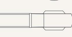
G1 = Spherical bearing, bore 16mm, model GS16
