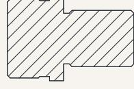
L1 = L shape, width 20mm, aperture 12.5mm
