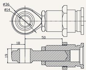
G1 = Spherical bearing, bore 16mm, model GS16
