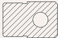
U1 = groove width 15.5mm, hole diameter 20.5mm
