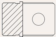
U2 = groove width 15.5mm, hole diameter 25.5mm
