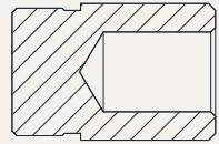
M2 = Type M, M30 thread, depth 20 mm
