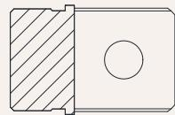
M1 = Type M, M25 thread, depth 20 mm
