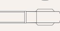
G1 = Spherical bearing, bore 30mm, model GS30
