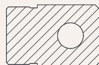
L2 = L shape, width 25mm, aperture 25.5mm
