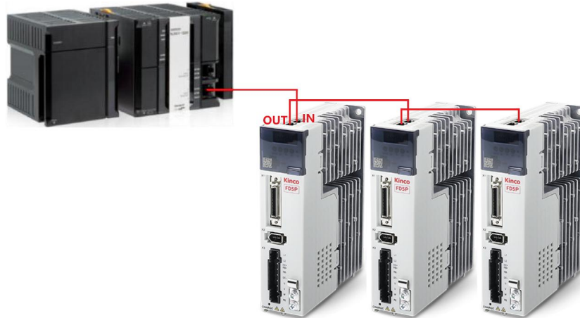
Figure 3-3 Omron NJ controller connecting drives
